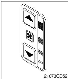
(1) It is possible to control the fan to four steps.
