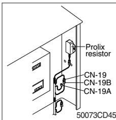
(1) This resistor is used to ensure continuous operation in case of a malfunction of the MCU.
