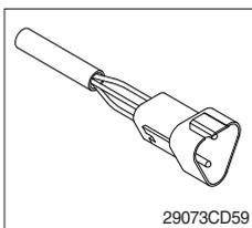
(1) The MCU communicates the machine data with a laptop computer through the RS232 connector.
