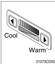
(1) There are 9 steps to control temperature from max cool to max warm controlled up and down by 1 step.
