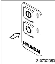
(1) Operating this switch turns the compressor and the LED simultaneously on or off.
