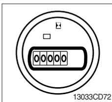
(1) This meter shows the total operation hours of the machine.
